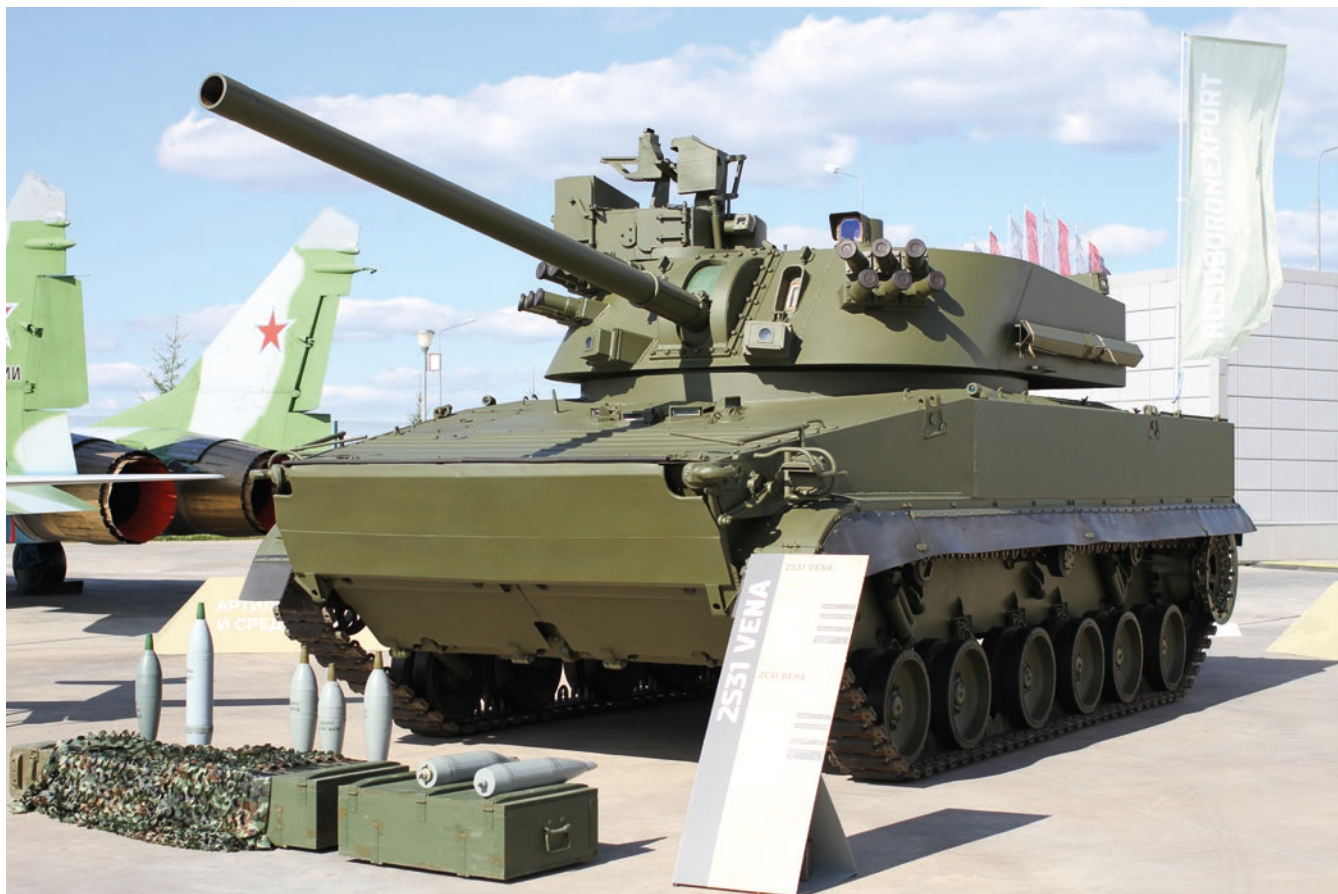
The Vena self-propelled gun can be used as a mortar (photo: Olga Korobkova)
